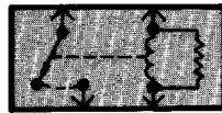
RELAY SHOWN WITH RESISTOR ACROSS COIL RESISTOR ACROSS COIL IS FOR NOISE SUPPRESSION
